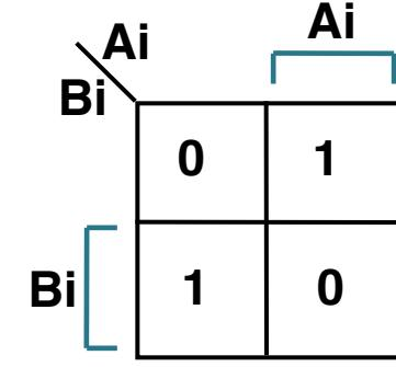
$$\begin{aligned}\text{Sum} &= \bar{A}_i B_i + A_i \bar{B}_i \\ &= A_i \oplus B_i\end{aligned}$$
